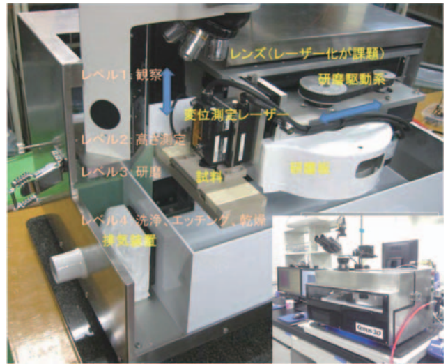
Fig.3 Fully automated 3D serial-sectioning microscope, Genus_3D™.
